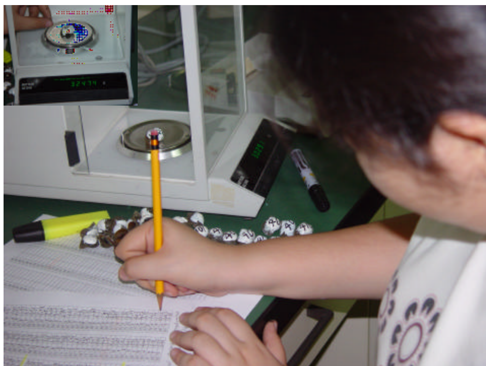
Plate 4. Weighing marked GAS individually in the Metler AE 240 digital balance.
